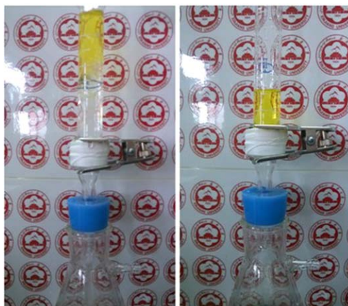
Figure 5. The separation of the hydrogel-coated mesh for oil-water mixtures, and the separation efficiency for each mixture (black is semi-IPN; gray is IPN). [Color figure can be viewed in the online issue, which is available at wileyonlinelibrary.com .]
